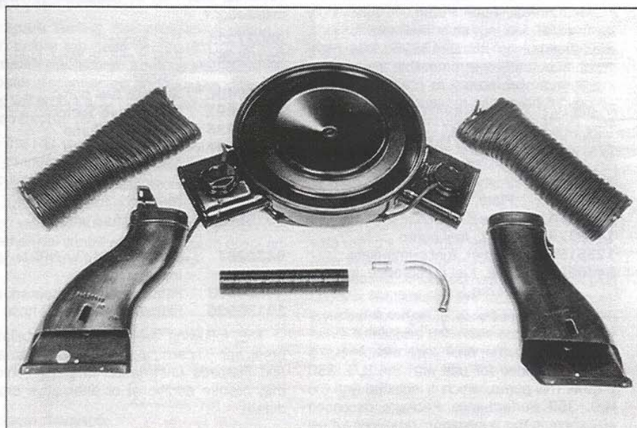
A dual-snorkel air cleaner assembly from a 1983-86 L69 Camaro can be adapted to other vehicles for improved off-highway performance with a Quadrajet-equipped H.O. 350 engine.
