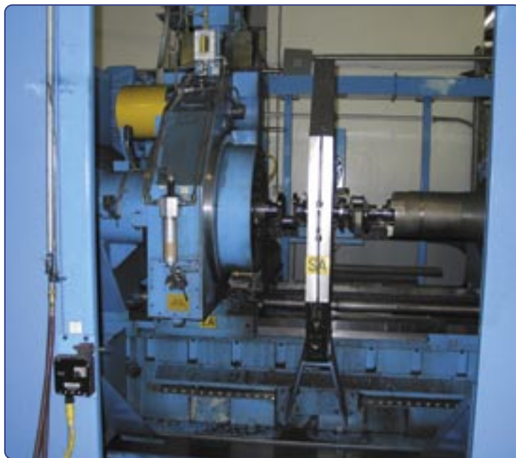
This is one of two American GFM crankshaft milling machines. This is the machine that is the centerpiece for our crankshaft machining capability and is one of 30 CNC machining centers utilized at SCAT.
