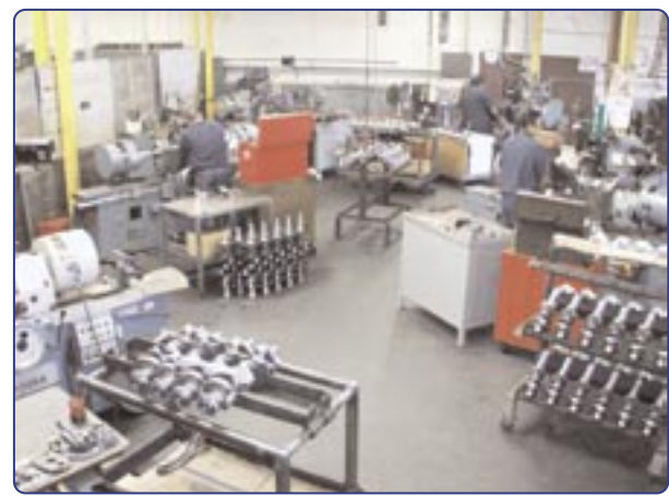
SCAT has new crankshaft grinding machines that are a key ingredient to ensuring our crankshafts meet our tight tolerances. Here, our skilled craftsmen grind diameters to finish sizes – this is one of the most critical operations in the process. Precision grinding insures tight tolerances.
