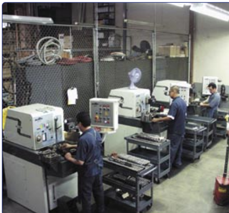
SCAT has 7 rod honing machines in our rod finishing department. We finish size our rods with our specialized diamond tooled machines and balance all our rods in house to the tightest tolerances in the industry.
