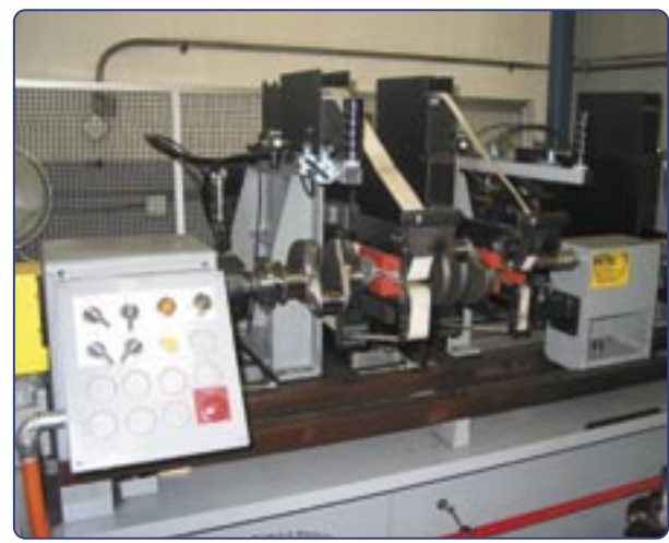
The final step in manufacturing a crankshaft is the polishing and inspection operations. SCAT has 6 polishing machines and our latest addition is a multi-arm automated polisher that ensures quality polishing and that the finish on the crankshaft is RA8 or better.
